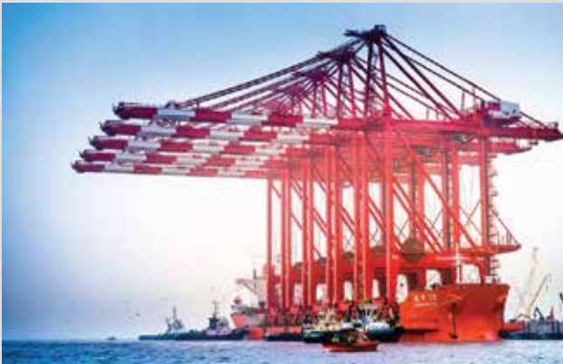
The ship-to-shore (STS) megamax quay cranes arriving in the Mersey in November 2015
