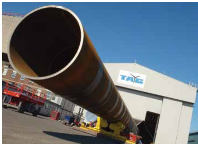
Monopile leaving TAG factory
