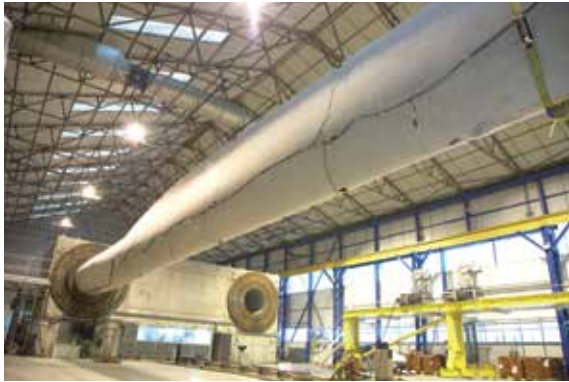
NAREC 100m blade test facility Courtesy of National Renewable Energy Centre
