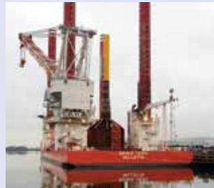
Top left: Keystone Engineering's twisted jacket Middle: Universal Foundation suction bucket on jackup Top right: FLIDAR at Gwynt y Môr
