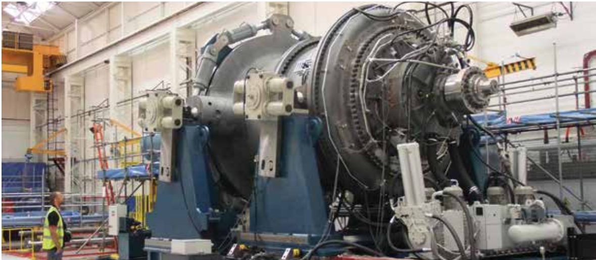
David Brown Wind's 7MW offshore gearbox under test
